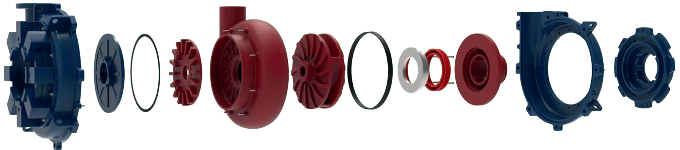
Assembly view of our slurryMAX™ pump major components
